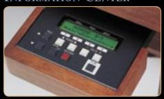
The drawbars, control tablets and rotary controls affect the operations necessary for performance on the organ. Advanced features such as drawbar voice mode, pedal sustain length etc., are accessed using the Information Center. This allows the player to see and make changes. The Information Center Display and touch buttons are located on a drawer unit positioned under the right side of the lower manual.
