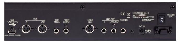
The back offers what can be expected from a stage organ. Along with headphone, line in and line out jacks, there is also an 8-pin Leslie output that can be used to connect an 8-pin Leslie cabinet or a Hammond adapter for other types of connector.
