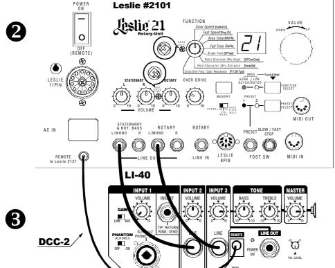
Make the connection shown in the figure at the left. Connect the Rotary-Unit to the Stationary-Unit using the DCC-2 Cable. Then connect the sound source to the LINE IN jacks as shown. Finally, connect the Stationary-Unit to AC power.
