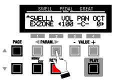
Notice that the number just underneath the word VOL is flashing "on" and "off."
