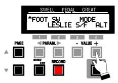
Notice that the legend on the bottom line of the display is flashing "on" and "off."
