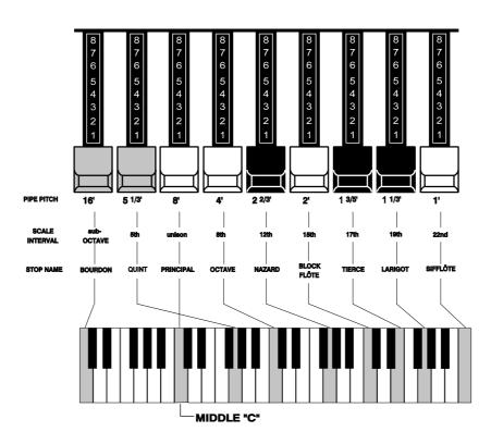
Each Drawbar is marked with a number followed by a footage mark. For example, the first white Drawbar is marked "8'." This is pipe organ terminology indicating that the pipe used to produce the lowest note on the keyboard on a pipe organ is actually eight feet long. The numbers from "1" to "8" on each Drawbar represent degrees of loudness – number 1 being the softest, and number 8 being the loudest.
