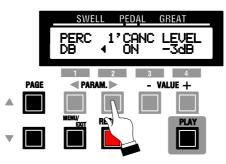
Notice that the legend just under the word LEVEL is flashing "on" and "off."
