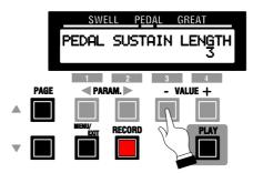
Notice that the number just underneath the word LENGTH is flashing "on" and "off."
