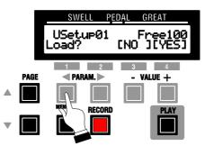
If the Card contains more than one Setup use the PAGE Touch Buttons to select the Setup containing the Preset Data you want.
