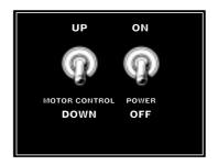
The second "toggle" switch is the **ON / OFF Power Switch**. To turn the organ "ON", simply push this switch forward so that it is in the "ON" position. After about 5 seconds, the organ will be ready to play. However, if you are using a Leslie Speaker cabinet with a tube amplifier, wait about 20 seconds until the tubes warm up.
