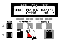
Notice that the legend just underneath the word TRNSPSE is flashing "on" and "off."
