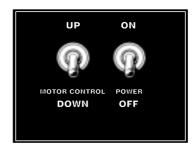
The second of these switches is the ON/OFF Power Switch and has already been explained. This is the equivalent of the RUN switch on the original Hammond Organs.
