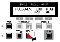
Notice that the legend underneath the word LOW is flashing "on" and "off."
