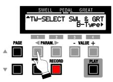
Notice that the legend <u>B-Type</u> is flashing "on" and "off."
