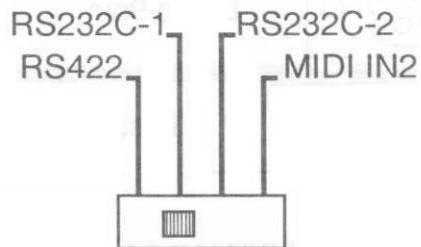
\* The Baud Rate of RS232C-1 is 31.25K (bit/sec.).
