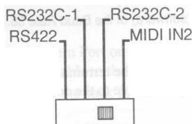
\* The Baud Rate of RS232C-2 is 38.4K (bit/sec.).
