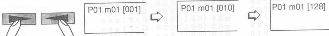
If you press the right arrow button while pressing the left arrow button, [ Instrument ] number moves about 10 times faster and stops at 128.
