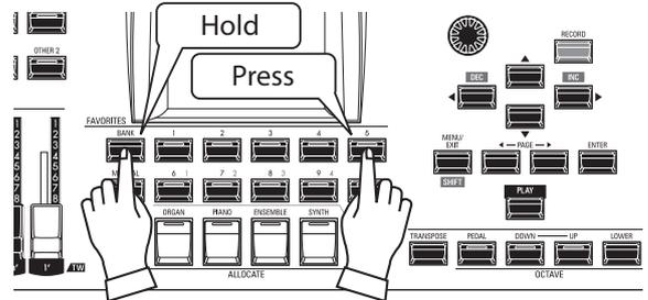
Press and Hold the [BANK] button and press the numbered [FAVORITE] button representing the Bank where the Combination you want to stored. The LED of the [FAVORITE] button will flash several times.
