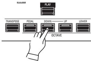
To change the Octave of the entire Keyboard (all Sections), press the OCTAVE [UP] or [DOWN] button. The display will show the current Octave setting.
