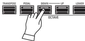
To change the Octave for the PIANO Section only, use the [DIRECTION] buttons to move the cursor to “PLAY Mode - PIANO Section - OCTAVE” and use the [VALUE] knob to change the Octave. The display will show the current Octave setting.
