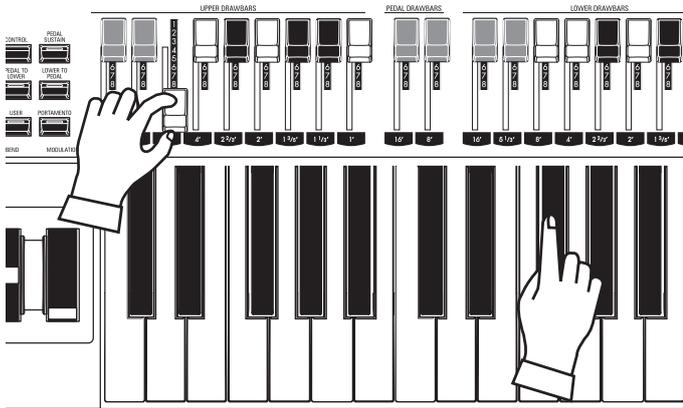
The Drawbars control the basic organ sounds. You can hear the effect each Drawbar has on the sound by pulling out or pushing in Drawbars while holding keys.
