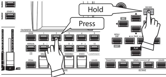
Select a Favorite Number. For this example, Press and Hold the red [RECORD] button and press the [FAVORITE] [2] button. The LED of the numbered button will flash several times. When the LED stops flashing the procedure is complete and your Bank is selected.
