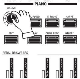
Use the [VOLUME] knob in the PIANO or ENSEMBLE Section to adjust the volume of the selected Section. For this example, use the [VOLUME] knob in the PIANO Section.
