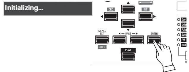
Use the [DIRECTION] [▼] button to move the cursor to the [INITIALIZE] icon, and press the [ENTER] button. The screen will display “Initializing...” for approximately 1 second.
