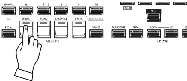
Press the [ORGAN] button in the [ALLOCATE] button group “ON.” The LED will light and the ORGAN Section will play from the UPPER keyboard.
