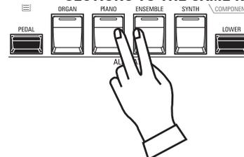
Press the desired Section buttons simultaneously. The above figure shows switching on both PIANO and ENSEMBLE Sections.
