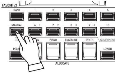
Normally, one of the [FAVORITE] buttons is “ON” (LED lit), indicating that a Combination has been selected. However, if you want to deselect Combinations and use the front panel controls entirely to control the sound, turn the [MANUAL] button “ON.” The [FAVORITE] buttons will all turn “OFF” and all sounds and features of the SKX PRO will be controlled by the front panel controls as well as by the Advanced Feature settings from the Menus.
