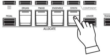
If the LED on the [SYNTH] button in the [ALLOCATE] button group is not “red,” press the [SYNTH] button. The LED will light red.
