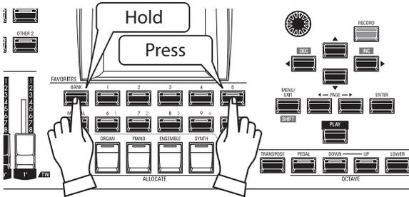
Select the Bank. For this example, select Bank 5. Press and Hold the [BANK] button and press the [5] [FAVORITE] button. The LED of the selected number will flash several times.
