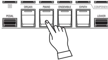
To play a PIANO or ENSEMBLE Patch on the UPPER keyboard, simply press the [PIANO] or [ENSEMBLE] button in the [ALLOCATE] button group. The LED will light red and the PIANO or ENSEMBLE Section in the display will be highlighted.
