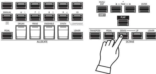
To change the Octave of the entire Keyboard (all Sections), press the OCTAVE [UP] or [DOWN] button. The display will show the current Octave setting.
