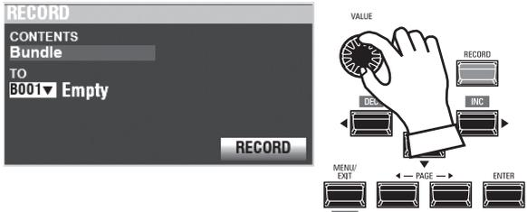
Use the [VALUE] knob to select the content to Record. For this example, select **Bundle**, which Records multiple contents simultaneously.
