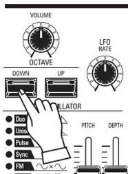
To change the Octave of the Oscillator, press the OCTAVE [UP] or [DOWN] buttons in the MONO SYNTH Section. The display will show the current Octave setting.
