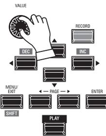
Use the [DIRECTION] buttons to move the cursor to “VEL,” and use the [VALUE] knob to select the Velocity Curve. The setting range is “Off” and “1” to “4.”
