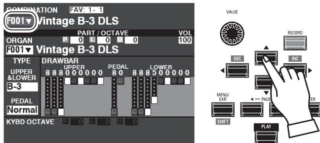
If the cursor is not at the Combination Number (very top of the screen), move the cursor to it using the [DIRECTION] buttons.
