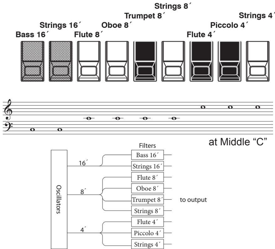
The figures to the left follow the layout of the Italian "Combo Compact" and the "TOP 7" combo organs, which used rocker-type tilt tablets rather than Drawbars to turn voices "ON" and "OFF". On the SKX PRO, the Drawbars are used to control the same sounds.
