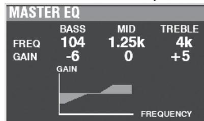
You can adjust the Master Equalizer Parameters by Press and Hold the [MASTER EQ] button and moving the AMPLITUDE ENVELOPE Slider Controls in the MONO SYNTH section (see the illustration at the top of this page).
