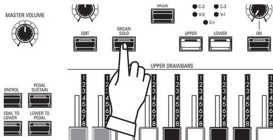
The ORGAN Section has 3 Parts - UPPER, LOWER and PEDAL. The [ORGAN SOLO] button turns all the Parts of the Organ Section “ON,” and turns other Sections “OFF.” This allows you to turn the SKX PRO into a vintage 2-keyboards-and-pedal Hammond Organ instantly with one button press.
