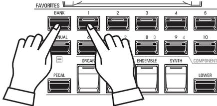
Press and Hold the [BANK] button and press a [NUMBER] button to select a “BANK.”
