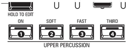
An important component of the Hammond Sound is “Touch-Response Percussion Control™.” The Percussion controls on the SKX PRO consist of four separate buttons (shown at left) which control harmonic Percussion tones. These four buttons control all the same functions as the tilt tablets on a Tone Wheel Hammond.
