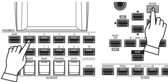
Press and Hold the [RECORD] button and press a [NUMBER] button to record as “NUMBER.” This is where your setting will be stored.
