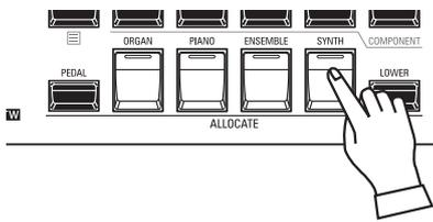
Press the [SYNTH] button in the [ALLOCATE] button group “ON.” The LED will light and the SYNTH Section will play from the UPPER keyboard.
