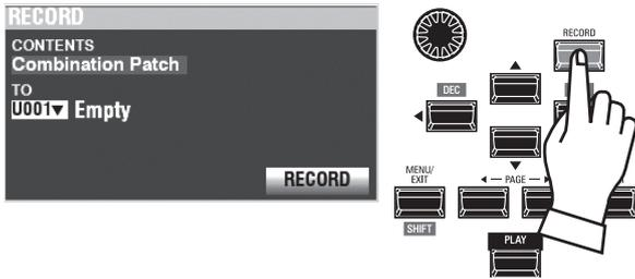
Press the red [RECORD] button at each Section or Combination page. The screen shown above will appear.
