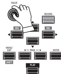
To change the Octave for the MONO SYNTH Section only, use the [DIRECTION] buttons to move the cursor to “PLAY Mode - MONO SYNTH Section - OCTAVE” and use the [VALUE] knob to change the Octave. The display will show the current Octave setting.
