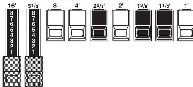
The two brown Drawbars on the far left give depth and richness to the sound. The left 16’ is one octave lower than the 8’, and 5 1/3’ is the third harmonic of the 16’ fundamental. Normally, the tones are built on the 8’ fundamental, but, if you want to add depth to the tone or to expand the playing range by one octave lower, build your tones on the 16’ fundamental.
