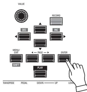
You can use the Patch List to display available Patches quickly. To open the Patch List, press the [ENTER] button when the Patch Number is highlighted in the display.
