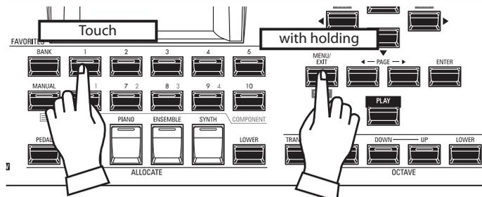
To display the Recorded Page, Press and Hold the [SHIFT] button and press the numbered [FAVORITE] button.
