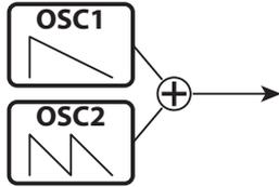
This setting utilizes two different pitched Oscillators. OSC1 sounds at “true pitch,” while OSC2 can be transposed up or down by one (1) octave in half-step increments. If the OSC2 LEVEL is set to “0,” only OSC1 will sound.
