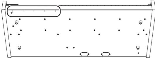
There are 5 mounting holes on the bottom of the instrument, allowing you to select one of 4 possible positions for the CU-1 switch.
