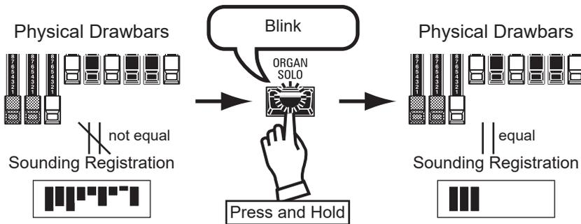
When you recall an ORGAN Patch, the Drawbar registration of the Recorded Patch is heard, instead of the physical Drawbar setting. If you move any Drawbar, its position takes precedence over the Recorded registration, although the Patch is not changed.
