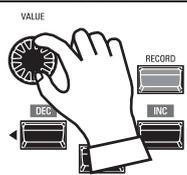
Use the VALUE Rotary Control to the right to raise the pitch. Use the VALUE Rotary Control to the left to lower the pitch.
