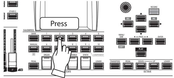
Press the numbered [FAVORITE] button where the Combination you want is stored. The LED of the numbered button will light and your Combination is selected.
