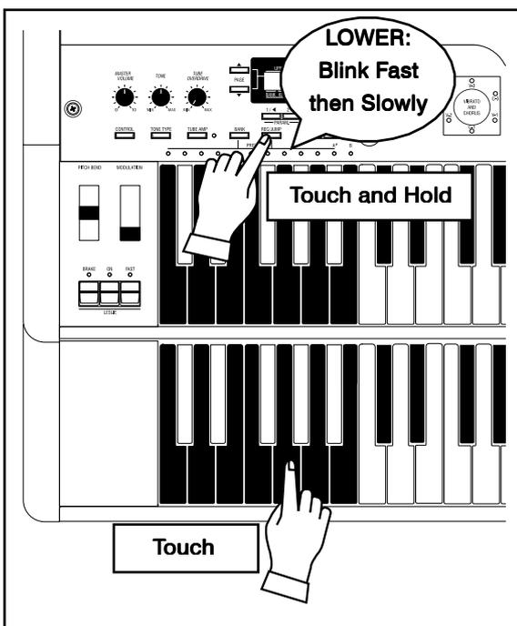
You can memorize the setting for only the LOWER and the PEDAL Parts for the XK-3 in the same BANK.
